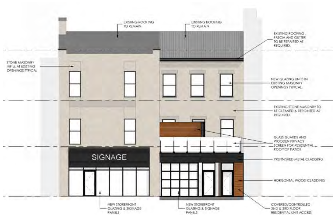
Figure 9: An elevation drawing of the Proposed alterations to the rear (South) façade of 35-37 & 39 Main St (EDGE Architects).
