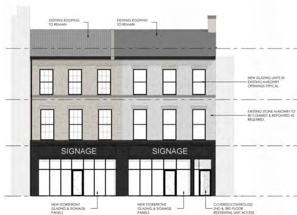
Figure 8: An elevation drawing of the Proposed alterations to the front (North) façade of 35-37 & 39 Main St (EDGE Architects).
