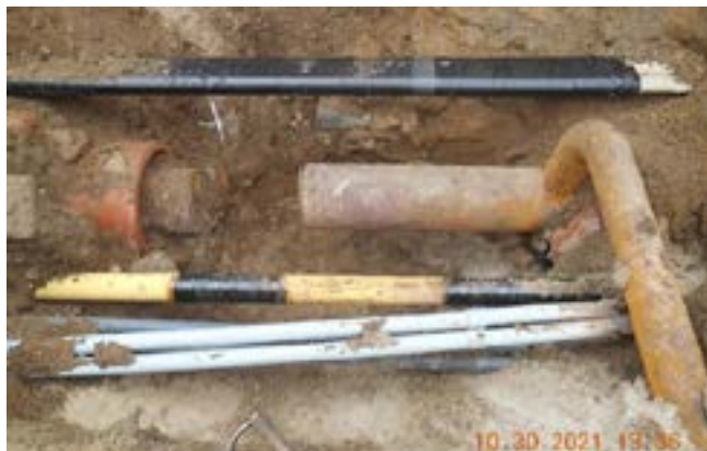
Defective underground piping.
