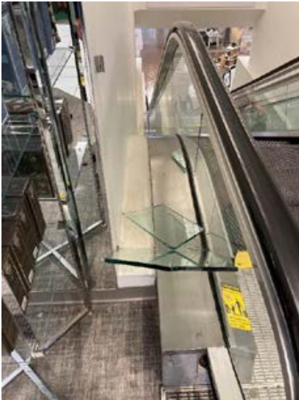
The glass shattered on impact with the rider's shoulder.
